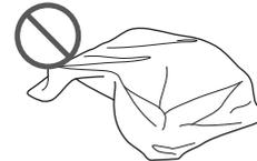
Do not block the ventilation holes (intake or exhaust)
