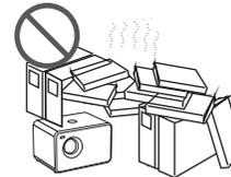
Do not install the projector in sites with improper ventilation.
