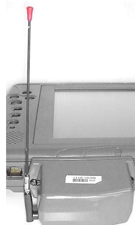
Antenna "Perpendicular" ("0 Degrees Landscape" Device User Orientation)
