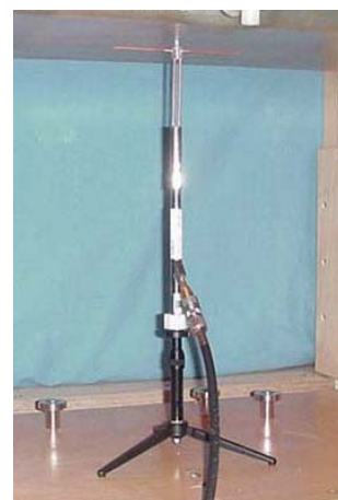
835MHz Dipole Setup
