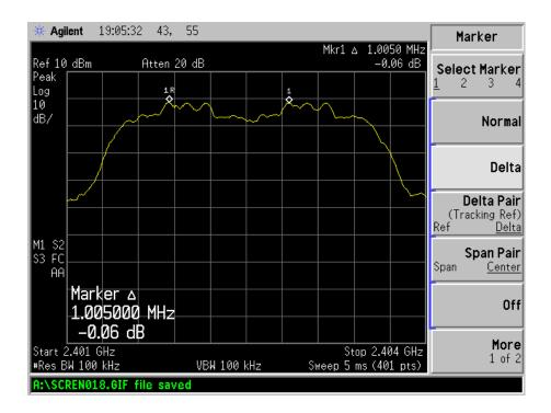
Channel Spacing (Middle CH=1MHz)
