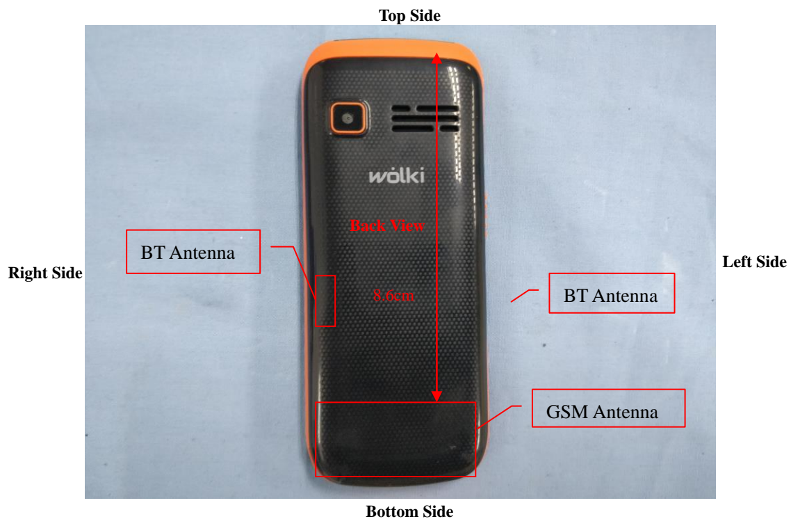
Block Diagram for EUT Antenna Position
