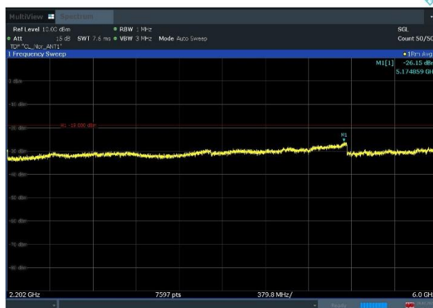
Plot 8-66. Conducted Spurious Emission Plot 2.202 GHz to 6 GHz (n66_2C_5M+20M_16QAM - Low Channel, Port 1)
