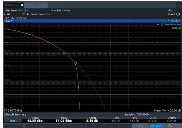
Plot 8-32. Peak To Average Power Ratio Plot (n70_1C_25M_16QAM-Mid Channel, Port 2)
