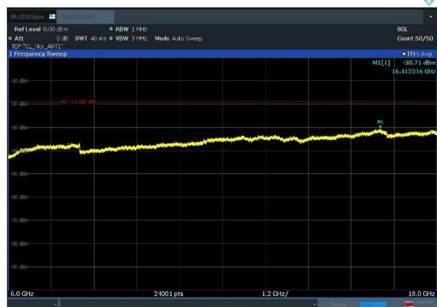
Plot 8-67. Conducted Spurious Emission Plot 6 GHz to 18 GHz (n66_2C_5M+20M_16QAM - Low Channel, Port 1)
