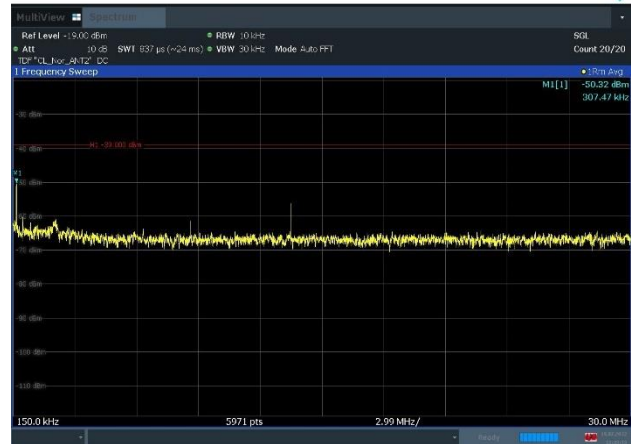
Plot 8-42. Conducted Spurious Emission Plot 150 kHz to 30 MHz (n66_1C_5M_16QAM - Low Channel, Port 2)
