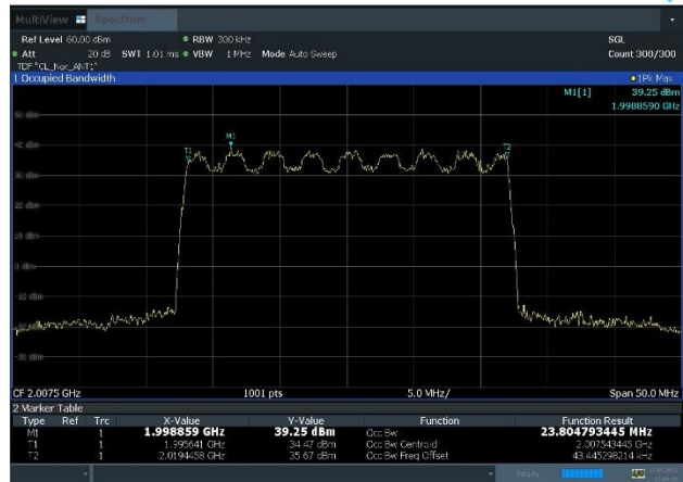
Plot 8-8. Occupied Bandwidth Plot (n70_1C_25M_16QAM - Mid Channel, Port 1)
