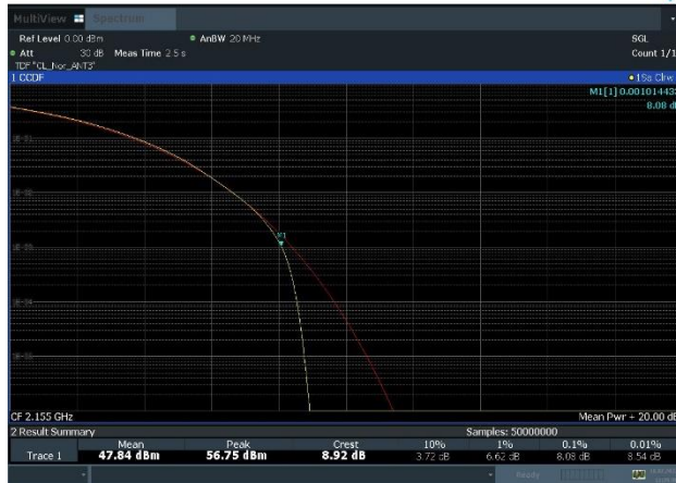
Plot 8-27. Peak To Average Power Ratio Plot (n66_1C_20M_QPSK - Mid Channel, Port 3)
