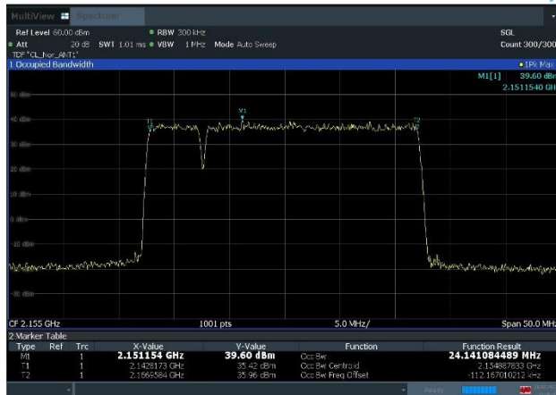
Plot 8-5. Occupied Bandwidth Plot (n66_2C_5M+20M_QPSK - Mid Channel, Port 1)
