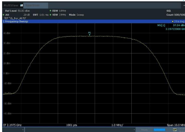
Plot 8-9. Power Spectral Density Plot (n66_1C_5M_16QAM - High Channel, Port 0)
