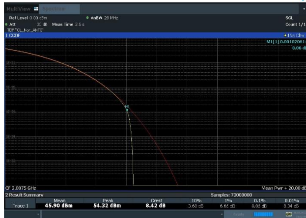
Plot 8-31. Peak To Average Power Ratio Plot (n70_1C_25M_QPSK-Mid Channel, Port 0)
