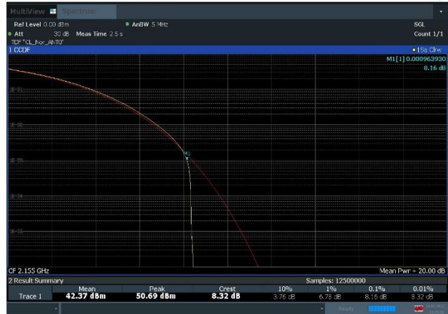
Plot 8-26. Peak To Average Power Ratio Plot (n66_1C_5M_64QAM - Mid Channel, Port 0)
