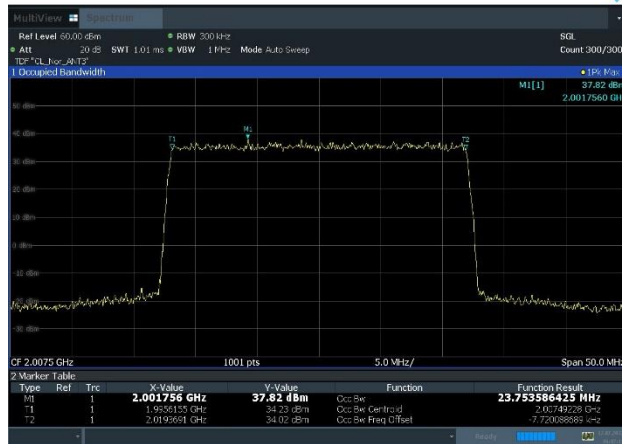
Plot 8-7. Occupied Bandwidth Plot (n70_1C_25M_QPSK - Mid Channel, Port 3)
