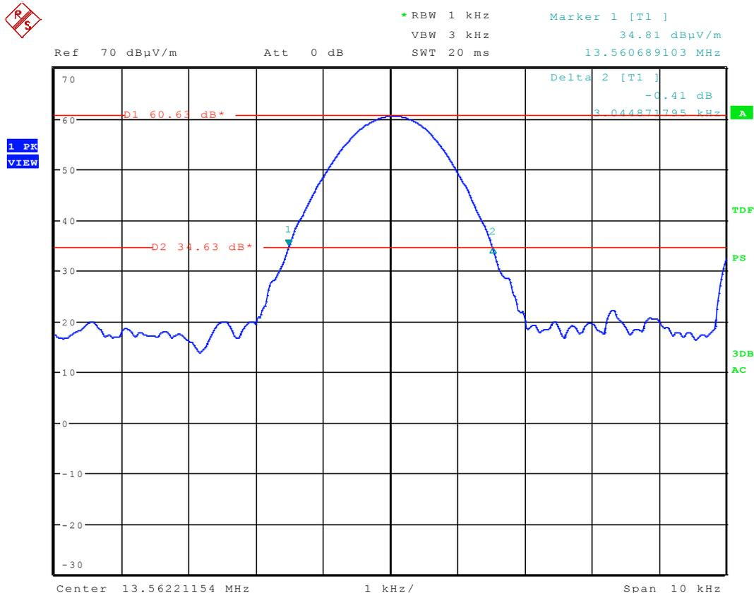
Occupied Bandwidth (-26 dB): **3.045 kHz**
