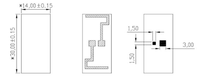
Figure 1 Physical dimension (mm)
