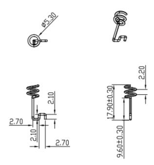
Figure 1 Physical dimension (mm)
