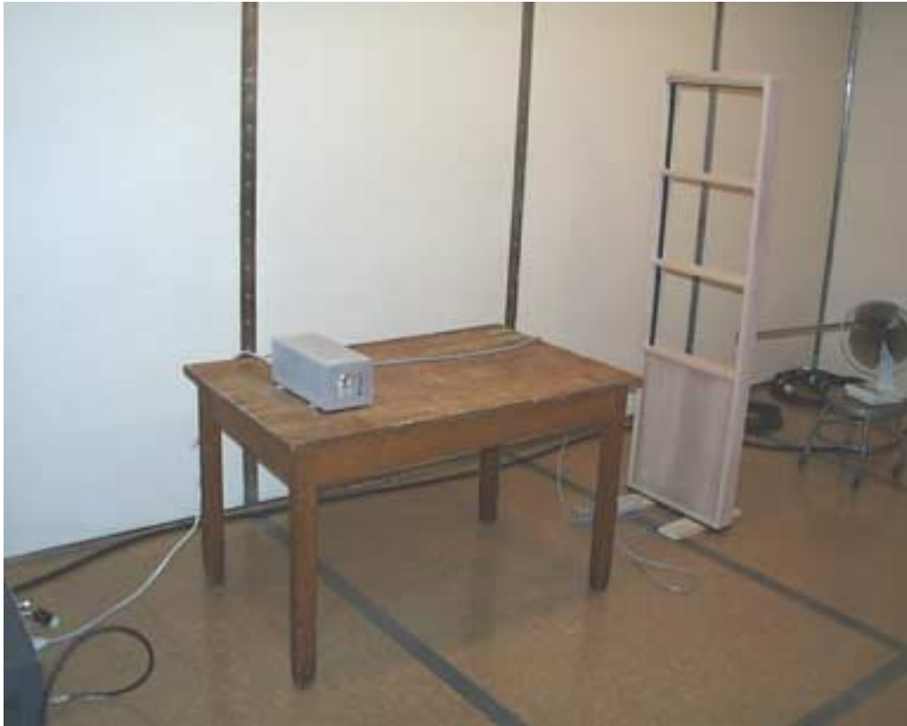
Photo 5 – Conducted Test Setup
