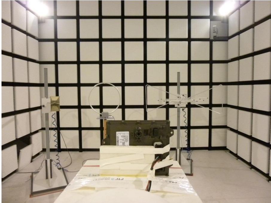
Photo 5: EUT at the anechoic chamber
