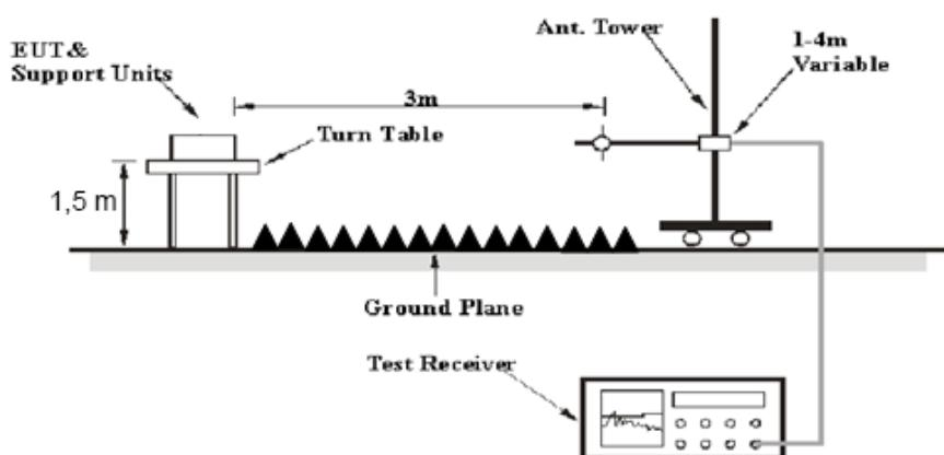
The radiated emission Below 1GHz tests were performed in the 3 meters chamber A, above 1GHz tests were performed in the 3 meters chamber B, using the setup accordance with the ANSI C63.10-2013. The specification used was the FCC 15.209, and FCC 15.247 limits and RSS-247 Clause 5.5, RSS-GEN Clause 8.10 limits.
