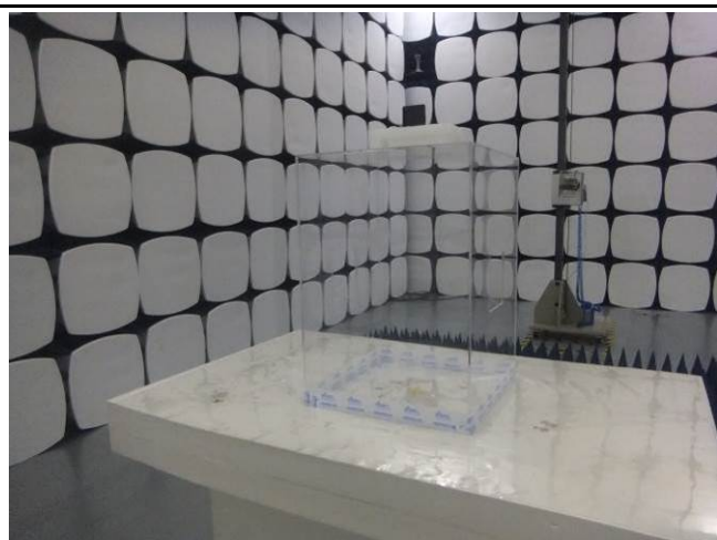
Radiated Spurious Emissions Test Setup Above 1GHz
