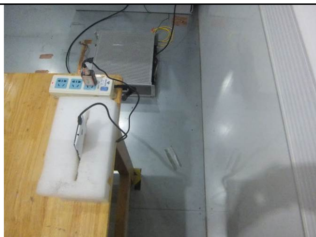
Conducted Emissions Test Setup Side View
