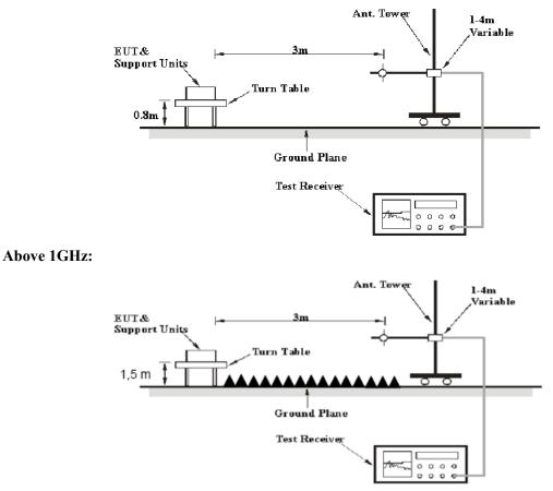
The radiated emissions were performed in the 3 meters distance, using the setup accordance with the ANSI C63.10-2013. The specification used was the FCC 15.209, and FCC 15.247 limits.
