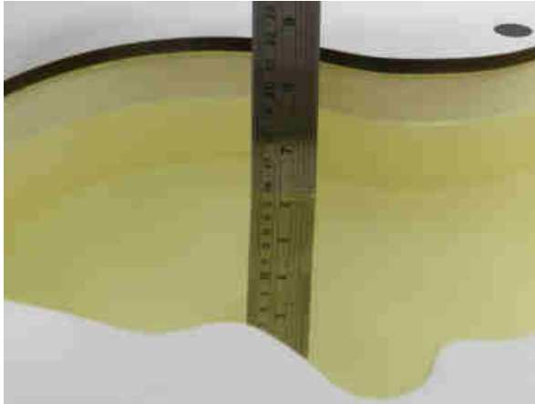
Fig 10.1 Photo of Liquid Height for Head SAR
