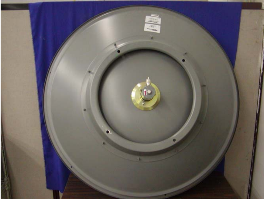
P3F-52-N7A Dish Antenna – Rear View
