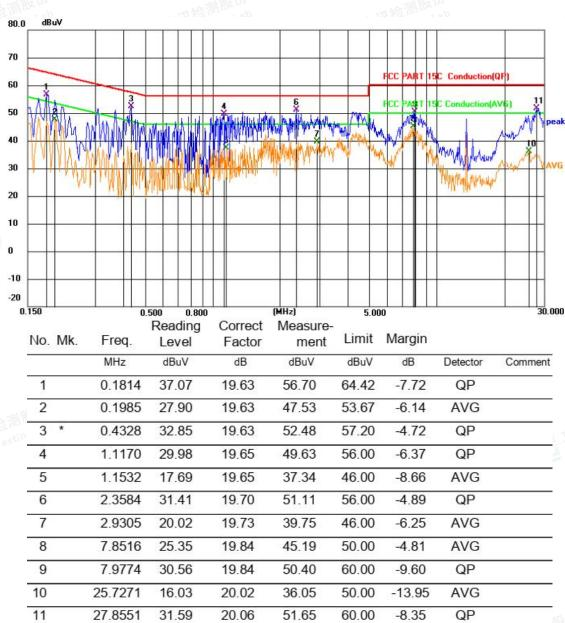
Measurement = Reading + Correct, Margin = Measurement - Limit.
