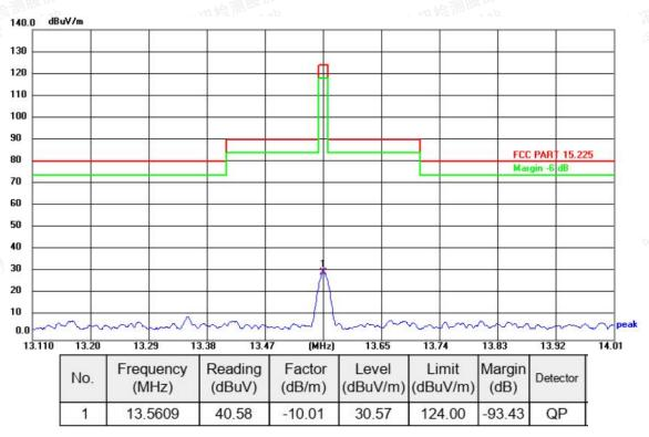
\*Note: Factor= Antenna Factor + Cable Loss
