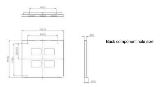
**NOTE** : The back component is installed and fixed using M6 expansion screws
