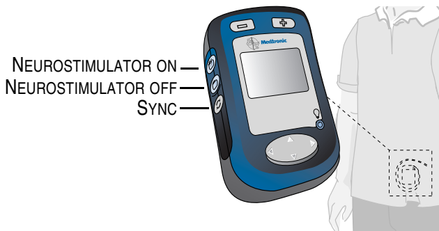
Figure 4.2 Synchronizing your neurostimulator and patient programmer.
