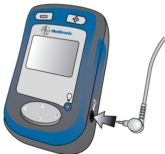
Figure 4.25 Insert the antenna plug into the antenna jack.
