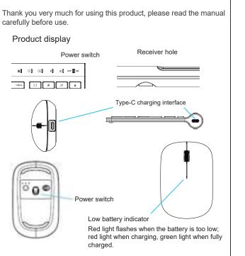
After the keyboard is powered on, the green light will turn on for 3S and then turn off
