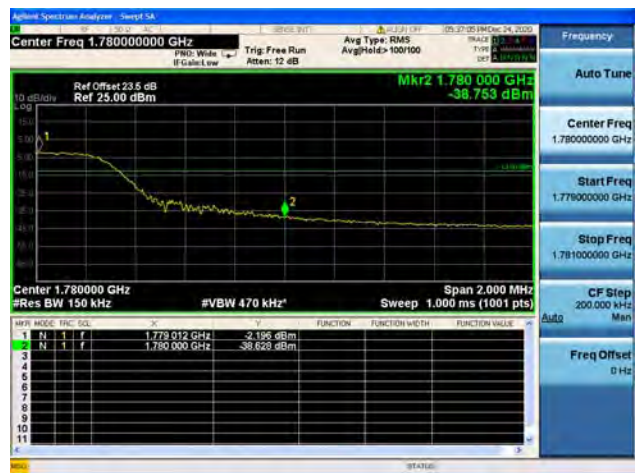
Band66 / 15MHz / High CH / QPSK / FULL RB
