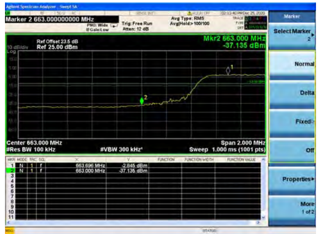
Band71 / 10MHz / High CH / QPSK / FULL RB
