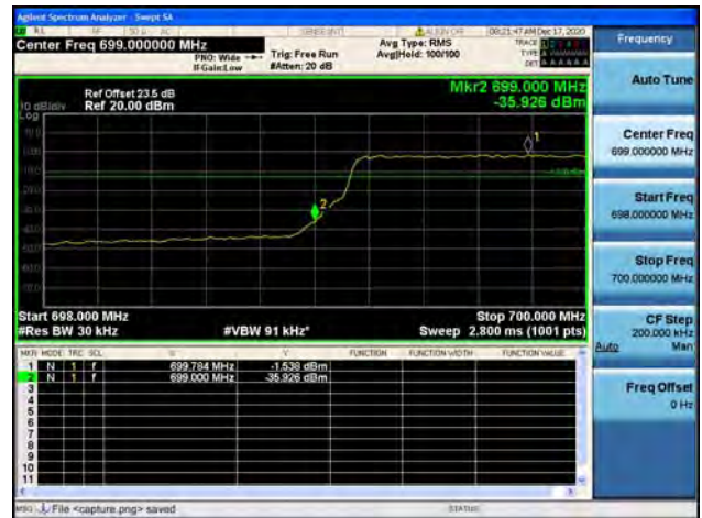
Band12 / 3MHz / High CH / QPSK / FULL RB
