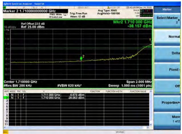
Band66 / 20MHz / High CH / QPSK / FULL RB
