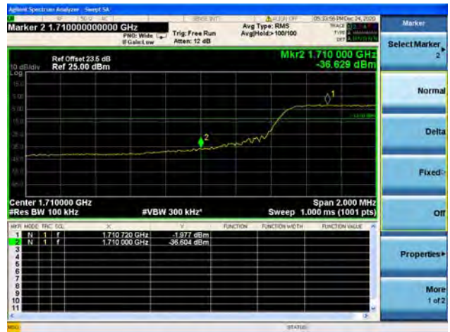
Band66 / 10MHz / High CH / QPSK / FULL RB
