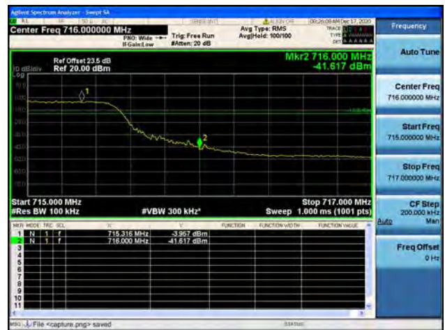
Band12 / 10MHz / High CH / QPSK / FULL RB
