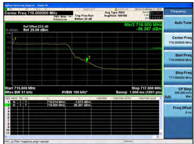
Band12 / 5MHz / High CH / QPSK / FULL RB
