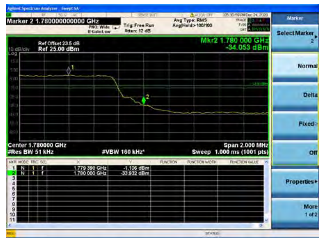
Band66 / 5MHz / High CH / QPSK / FULL RB
