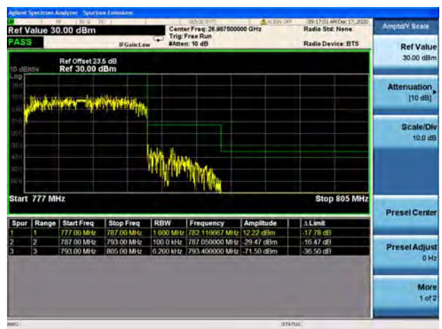
Band13 / 10MHz / High CH / QPSK / FULL RB
