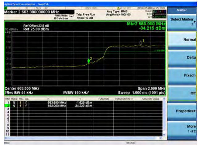
Band71 / 5MHz / High CH / QPSK / FULL RB
