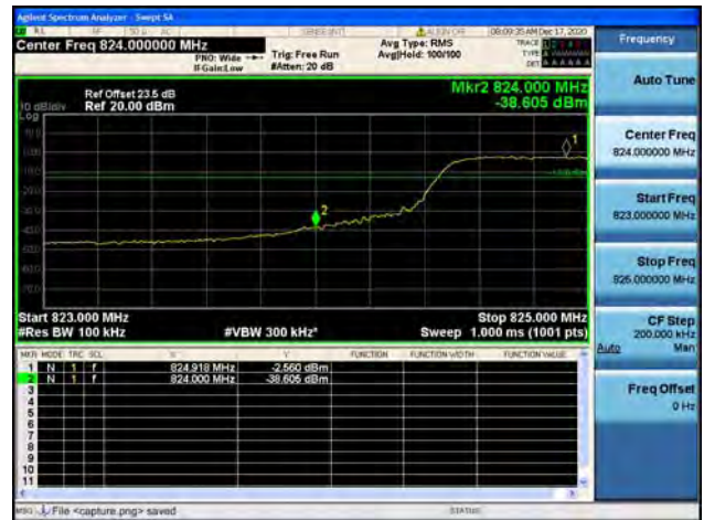
Band5 / 10MHz / High CH / QPSK / FULL RB
