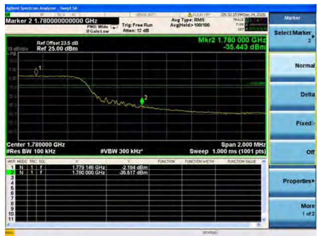
Band66 / 10MHz / High CH / QPSK / FULL RB
