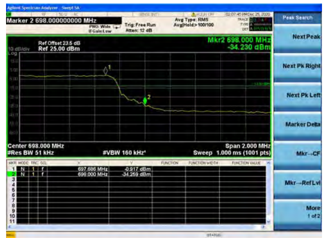
Band71 / 5MHz / High CH / QPSK / FULL RB
