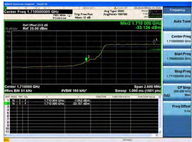
Band66 / 5MHz / High CH / QPSK / FULL RB
