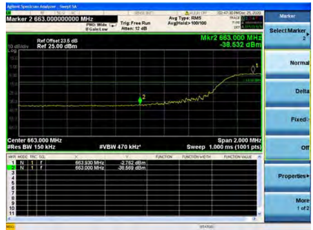
Band71 / 15MHz / High CH / QPSK / FULL RB
