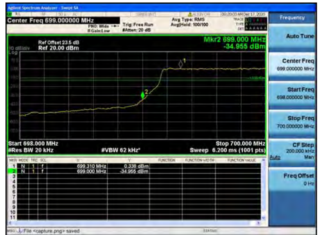
Band12 / 1.4MHz / High CH / QPSK / FULL RB
