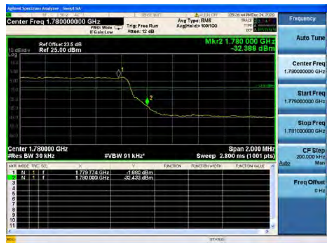
Band66 / 3MHz / High CH / QPSK / FULL RB
