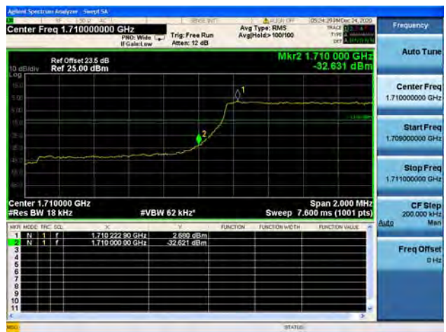
Band66 / 1.4MHz / High CH / QPSK / FULL RB
