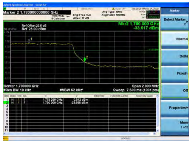
Band66 / 1.4MHz / High CH / QPSK / FULL RB
