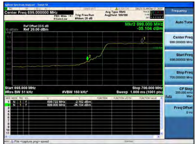
Band12 / 5MHz / High CH / QPSK / FULL RB
