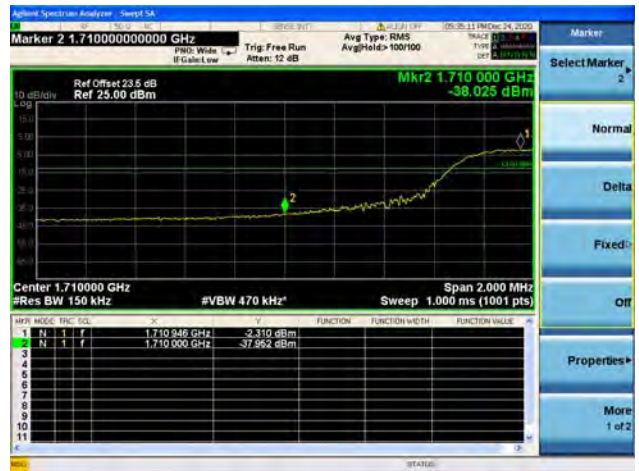
Band66 / 15MHz / High CH / QPSK / FULL RB
