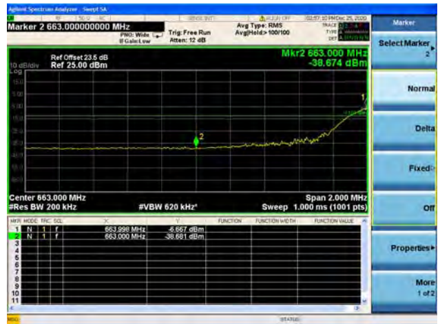
Band71 / 20MHz / High CH / QPSK / FULL RB
