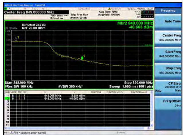
Band5 / 10MHz / High CH / QPSK / FULL RB
