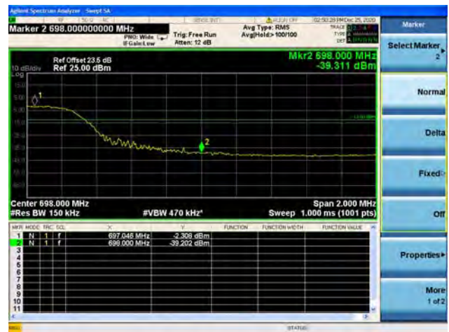
Band71 / 15MHz / High CH / QPSK / FULL RB
