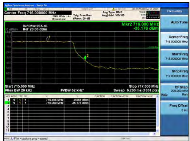
Band12 / 1.4MHz / High CH / QPSK / FULL RB
