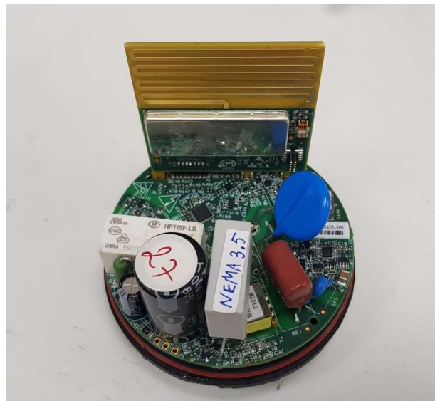
RF and Platform cards assembly
