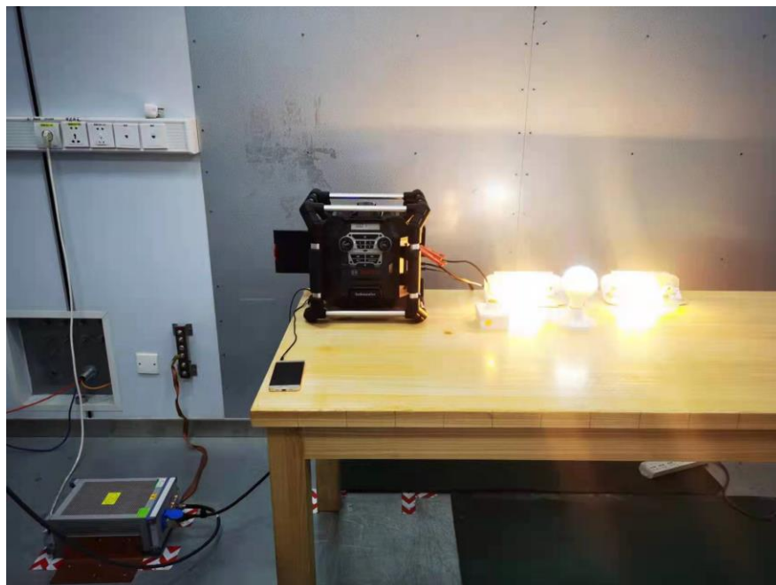
POWERLINE CONDUCTED EMISSIONS MEASUREMENT SETUP
