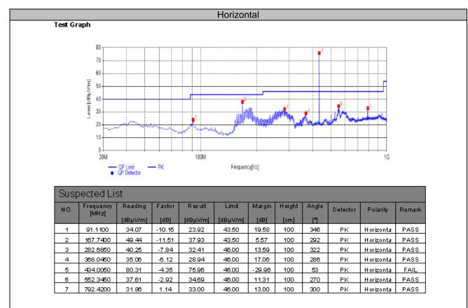
Note:1. Result (dB $\mu$ V/m) = Reading(dB $\mu$ V/m) + Factor (dB).
