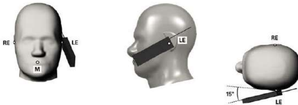
Fig.11.4 Illustration for Tilted Position
