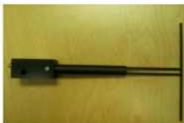
Figure 1 – MVG COMOSAR Validation Dipole
