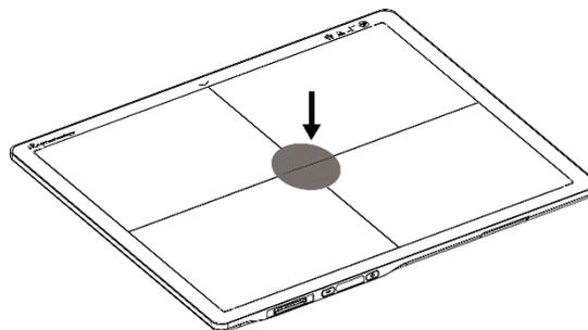
Local load: 100 kg on an area 4 cm in diameter
