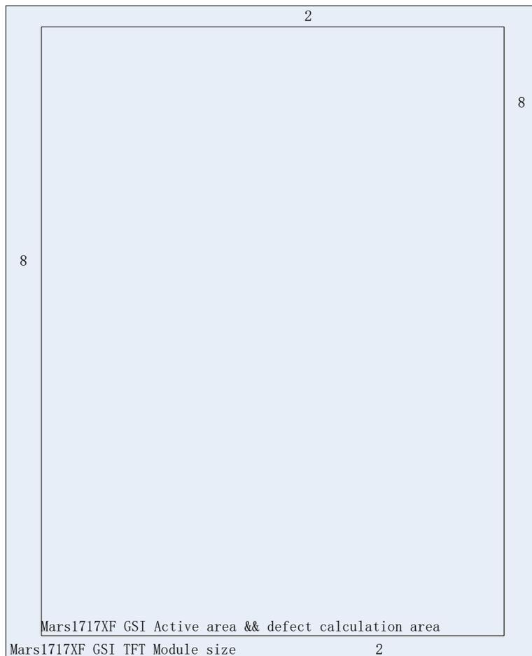
The Mars1717XF-CSI defect calculation area is 2826 x 2818, the active area is 2832 x 2836 and the TFT module size is 2848 x 2840
