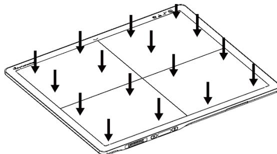
Uniform load: 150 kg over the whole area of the detector surface
