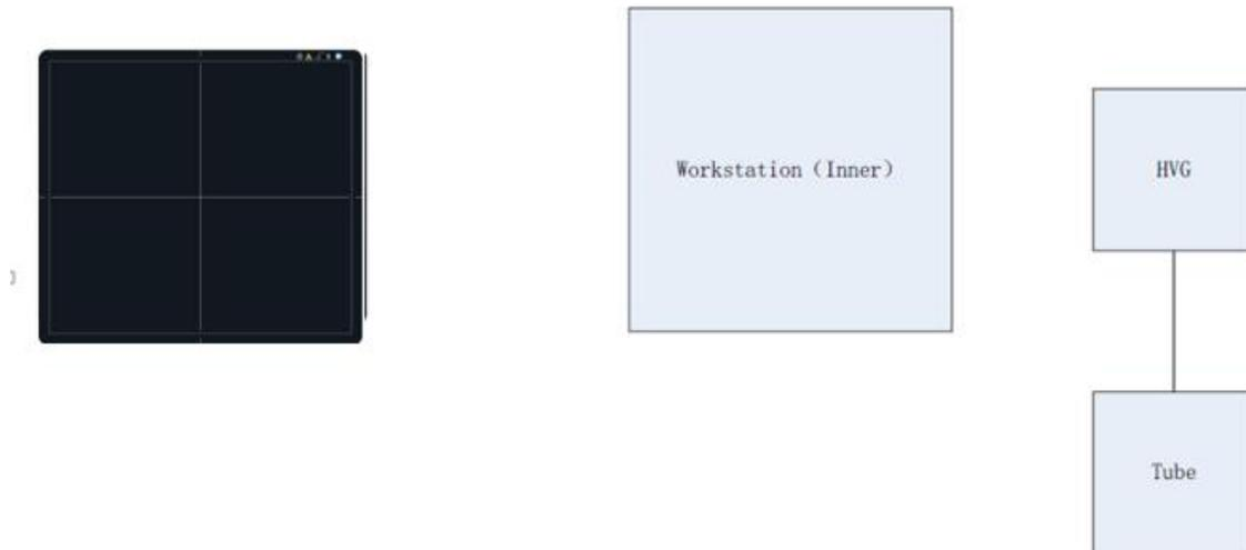
The workstation hosts the PC device installed with FDR SE Console or iDetector. Chapter 3.3 describes how to establish the connection between detectors and the workstation. In AED mode, the workstation does not control the X-ray generator; the user decides when to take the X-ray.
