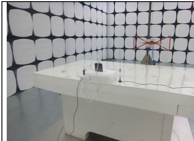
Radiated Spurious Emissions Test Setup Below 1GHz
