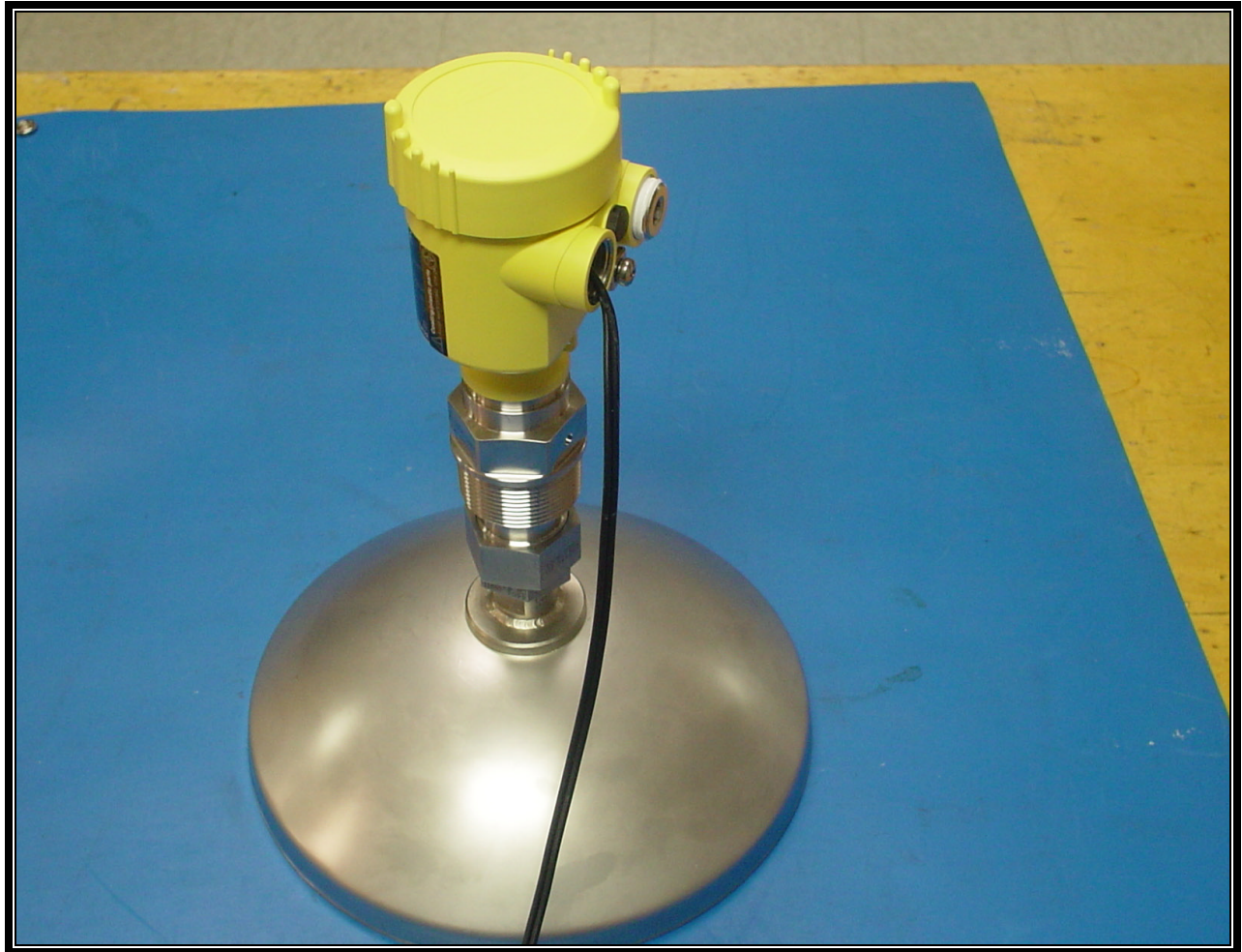
PHOTOGRAPH 5: EUT WITH 33 DBI PARABOLIC ANTENNA
