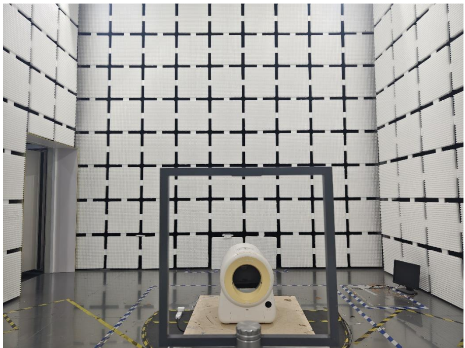
Radiation Emission Test Setup (Below 30MHz)
