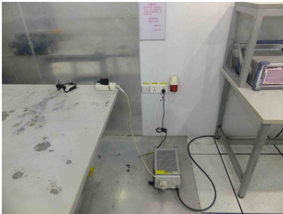
1 Photo of Power Line Conducted Emission Measurement
