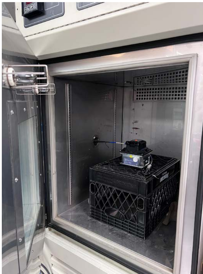
Figure 3.3 Frequency Tolerance Test Setup
