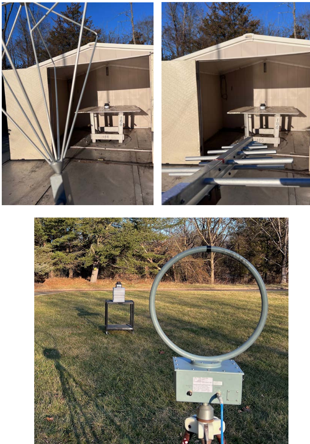
Figure 3.1 Radiated Emission Test Setup
