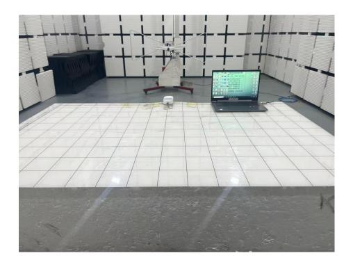
Set-up for Radiated Spurious Emission, Above 1GHz
