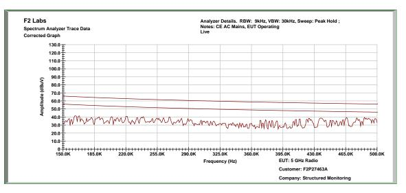
Conducted Test – Live: 0.5 MHz to 5.0 MHz
