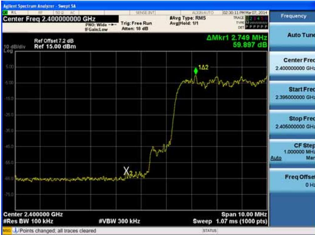
Test Plots with hopping (8DPSK)
