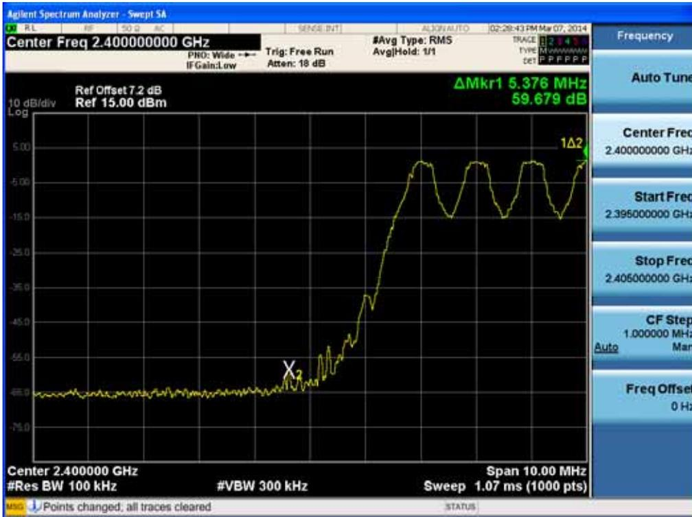
Test Plots with hopping (GFSK)
