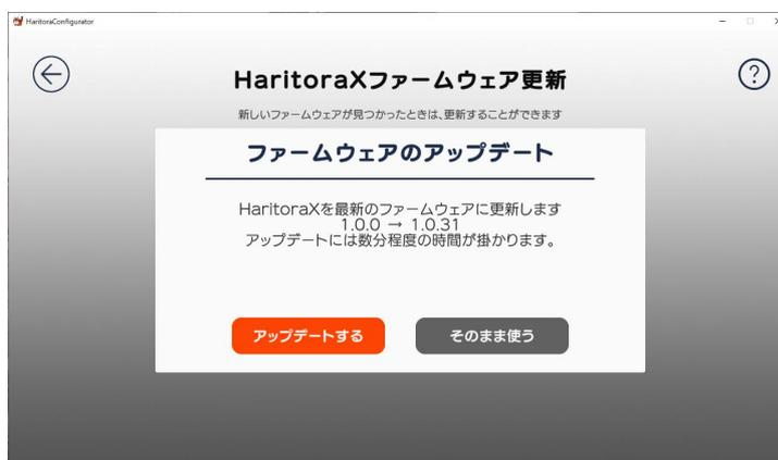
Select "Update" to update the firmware. After selecting, the LED of the main unit lights up so that three colors flow, and the gauge is displayed and the update starts. When the gauge reaches 100%, the update is complete.
