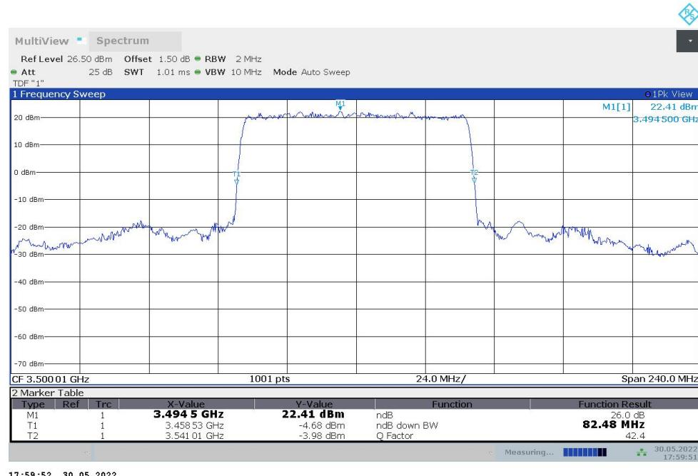
**n78L,80MHz Bandwidth,DFT-s-QPSK (-26dBc BW)**
