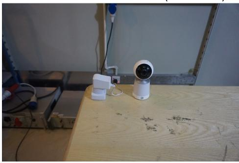
Radiated Emissions (30MHz-1GHz) Test Setup
