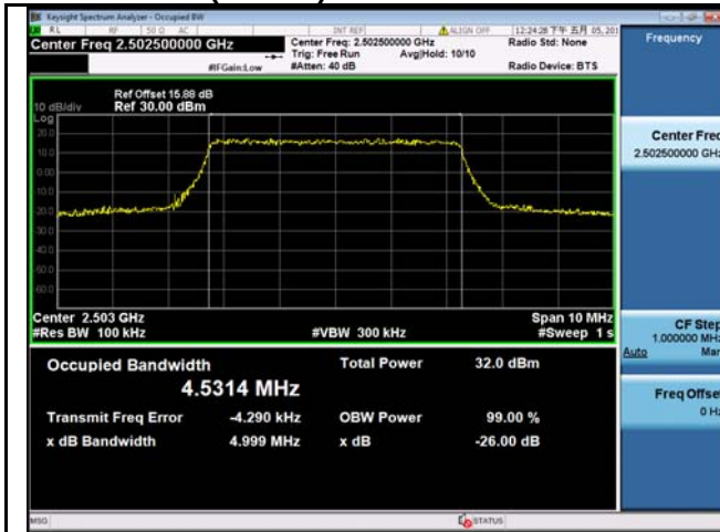
LTE band 7 - Low CH QPSK-5
