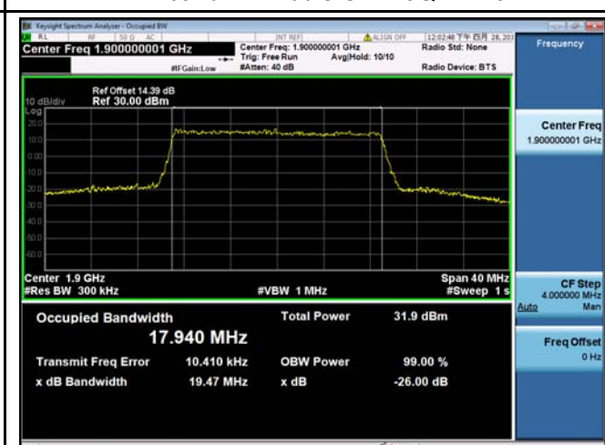
LTE band 2 - Middle CH 16QAM-20
