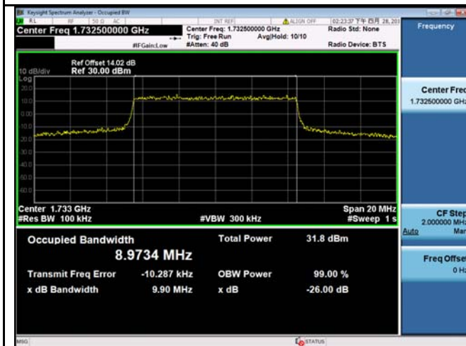
LTE band 4 - Low CH QPSK-10
