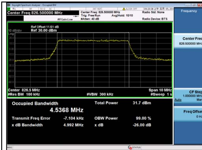
LTE band 5 - Low CH QPSK-5
