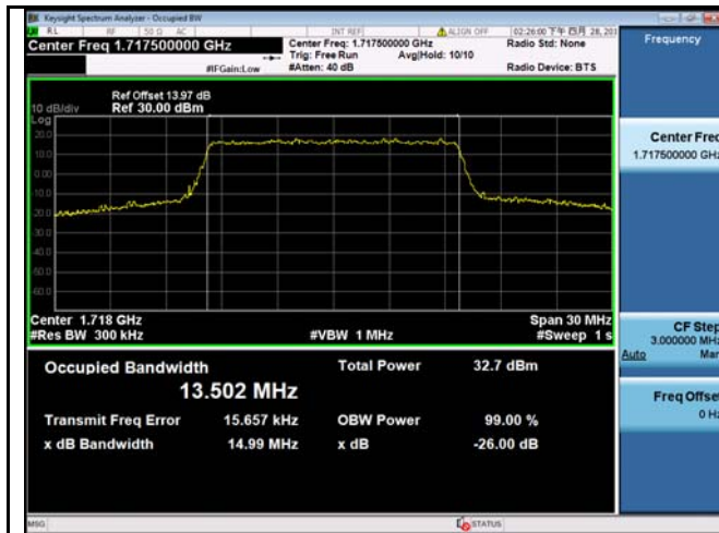
LTE band 4 - Low CH QPSK-15
