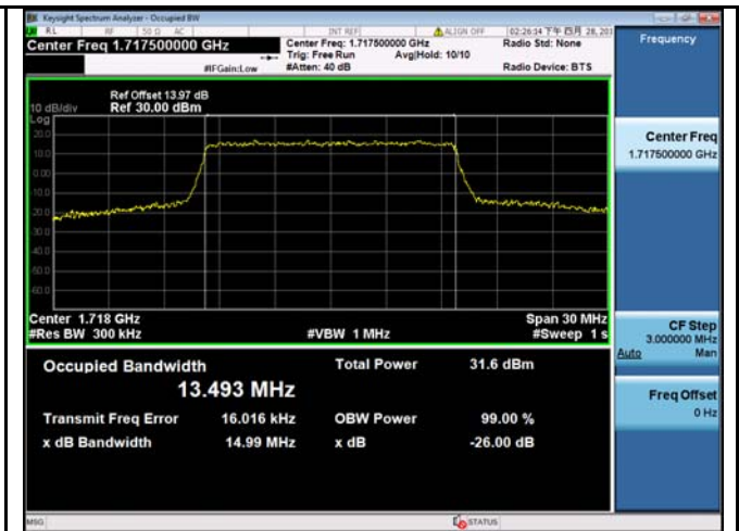
LTE band 4 - Low CH 16QAM-15
