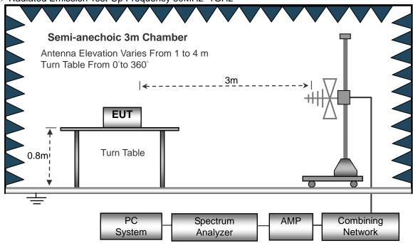
(C) Radiated Emission Test-Up Frequency Above 1GHz
