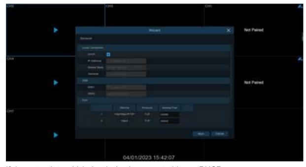
If the network to which the device is connected has a DHCP server, you can check the DHCP box, and the DHCP server will automatically assign all network parameters to the device. Alternatively, you can manually set the IP
