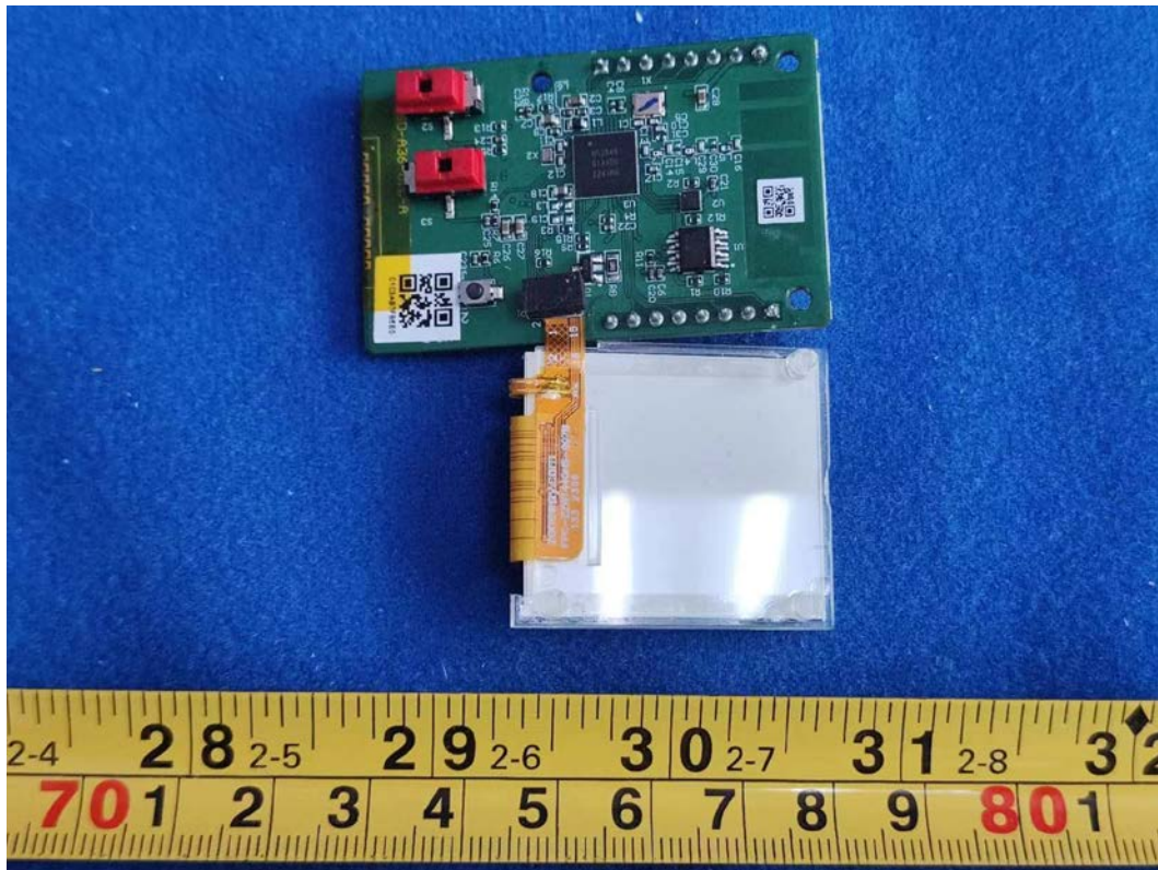
FIGURE 12 240 VAC 60 A WISER CONTROL RELAY (QO260PWX240) RF BOARD BACK
