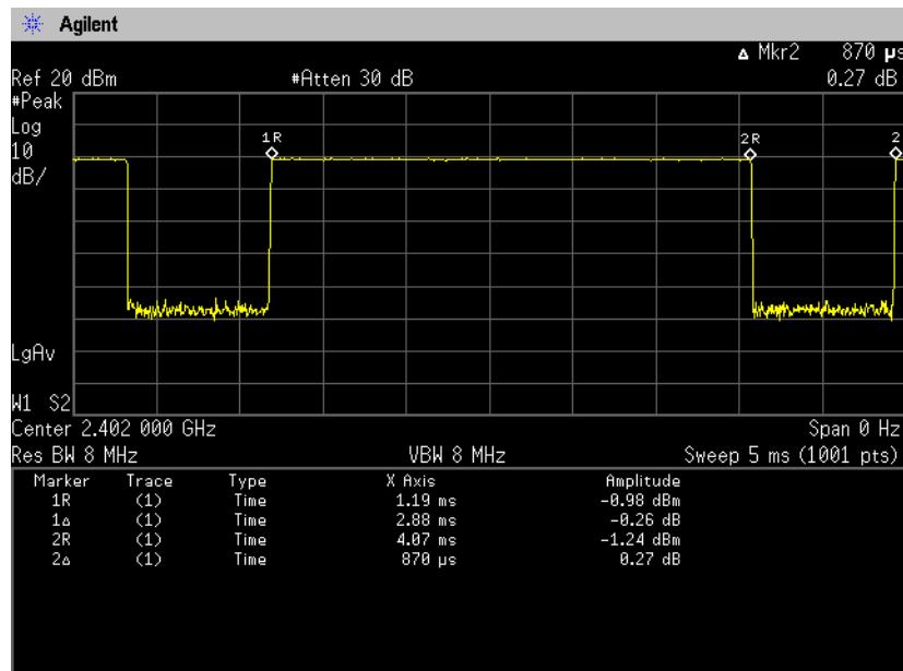
$$\text{Duty Cycle} = T_{\text{on}} / (T_{\text{on}} + T_{\text{off}}) = 2880[\text{us}] / (2880[\text{us}] + 870[\text{us}]) = 77.0[\%]$$
