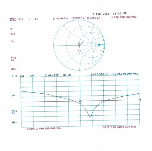
Impedance Measurement Plot for Head TSL
