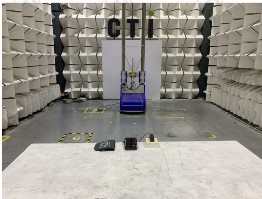
Radiated spurious emission Test Setup-1(Below 1GHz)
