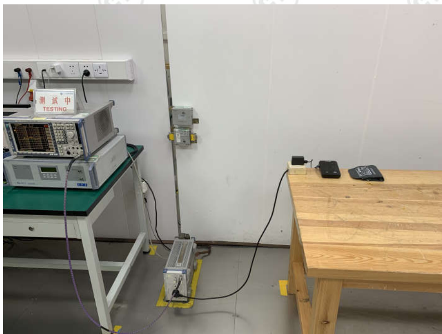
Conducted Emissions Test Setup
