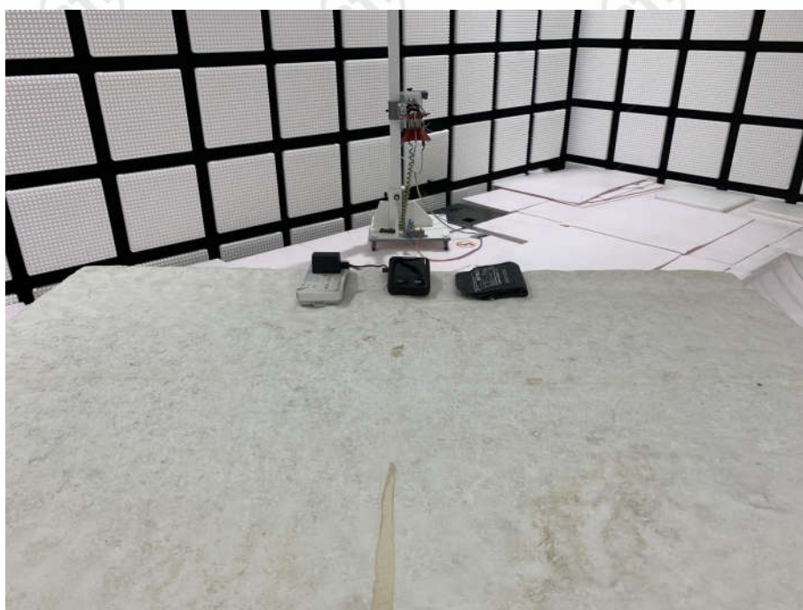
Radiated spurious emission Test Setup-2(Above 1GHz)
