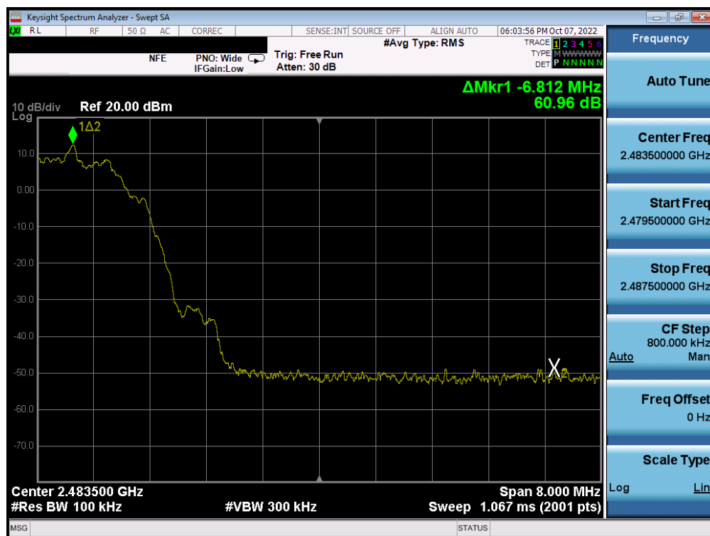
Plot 7-62. Band Edge Plot (Bluetooth (LE), 2Mbps - Ch. 39) - ANT 1
