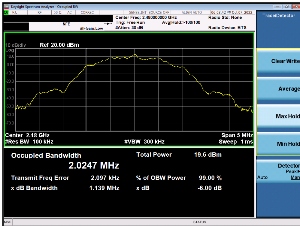
Plot 7-12. 6dB Bandwidth Plot (Bluetooth (LE), 2Mbps – Ch. 39) – ANT 1
