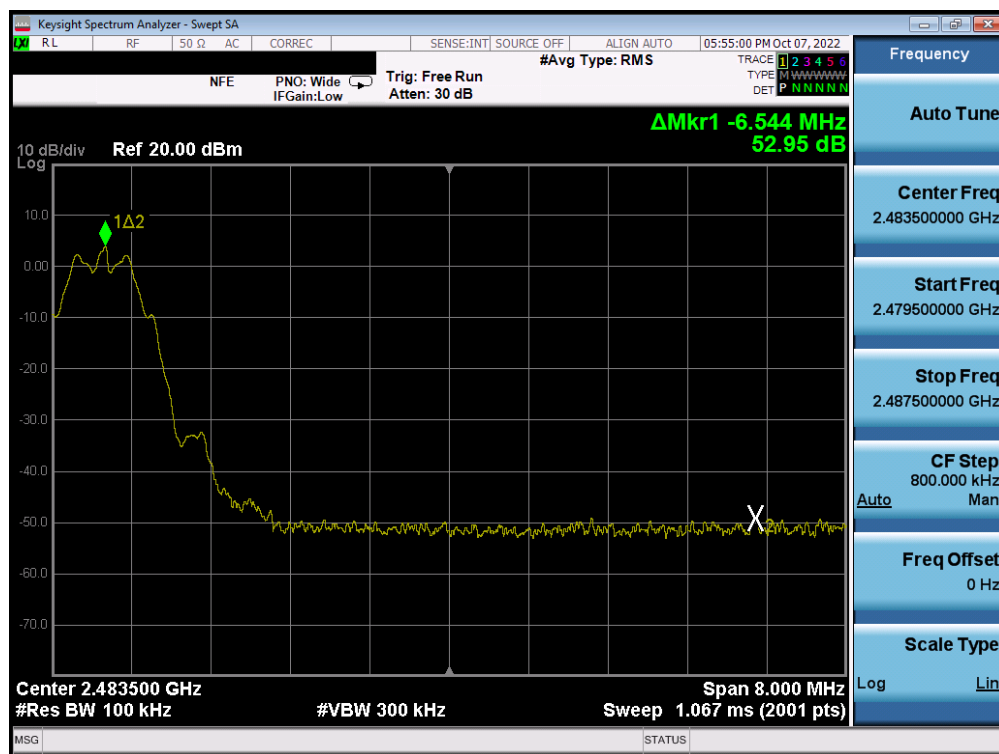
Plot 7-56. Band Edge Plot (Bluetooth (LE), 125kbps – Ch. 39) – ANT 1
