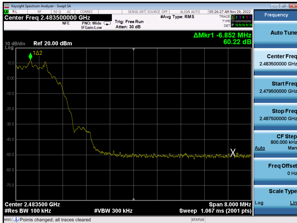
Plot 7-66. Band Edge Plot (Bluetooth (LE), 2Mbps – Ch. 39) – ANT 2
