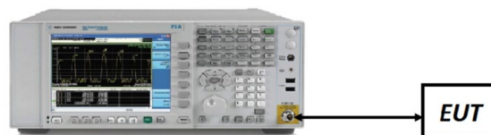
Figure 7-4. Test Instrument & Measurement Setup
