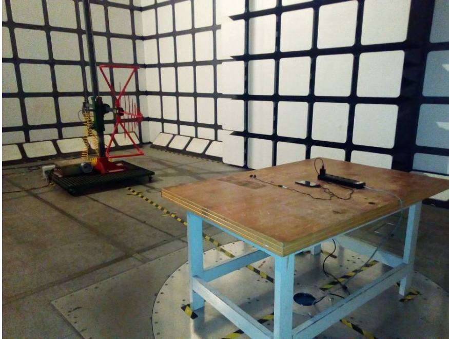
Radiated Emissions View (Below 1 GHz)
