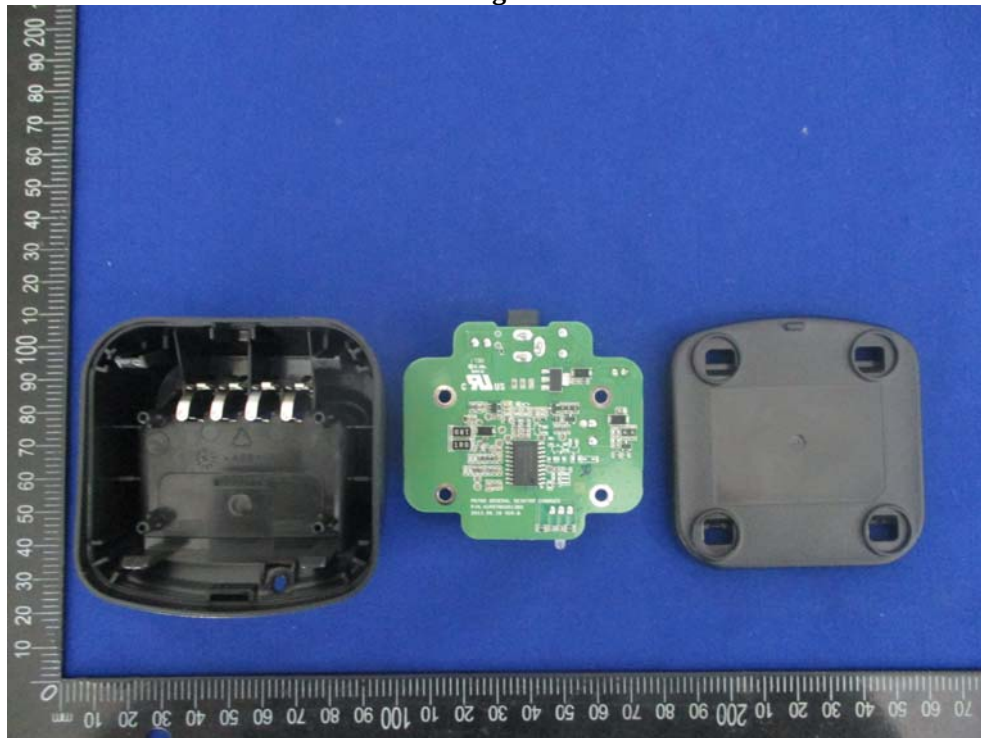
EUT –Base Charger Uncover View
