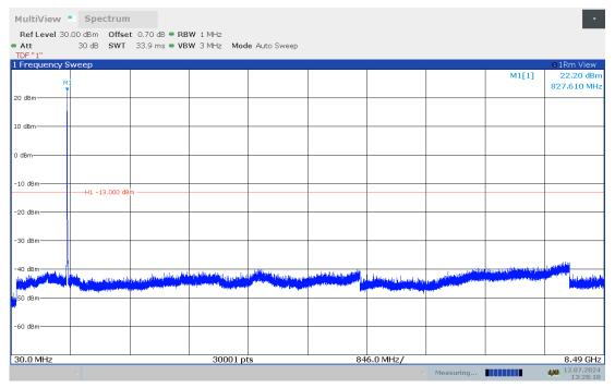
Channel 4183: 30MHz –8.49GHz Spurious emission limit –13dBm.
