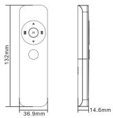
Note: The length L of the remote control depend on product specifications (unit: mm)
