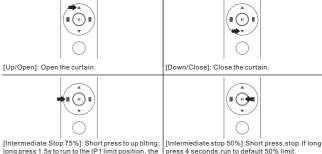
long press 1.5s to run to the IP1 limit position, the default is 75%
