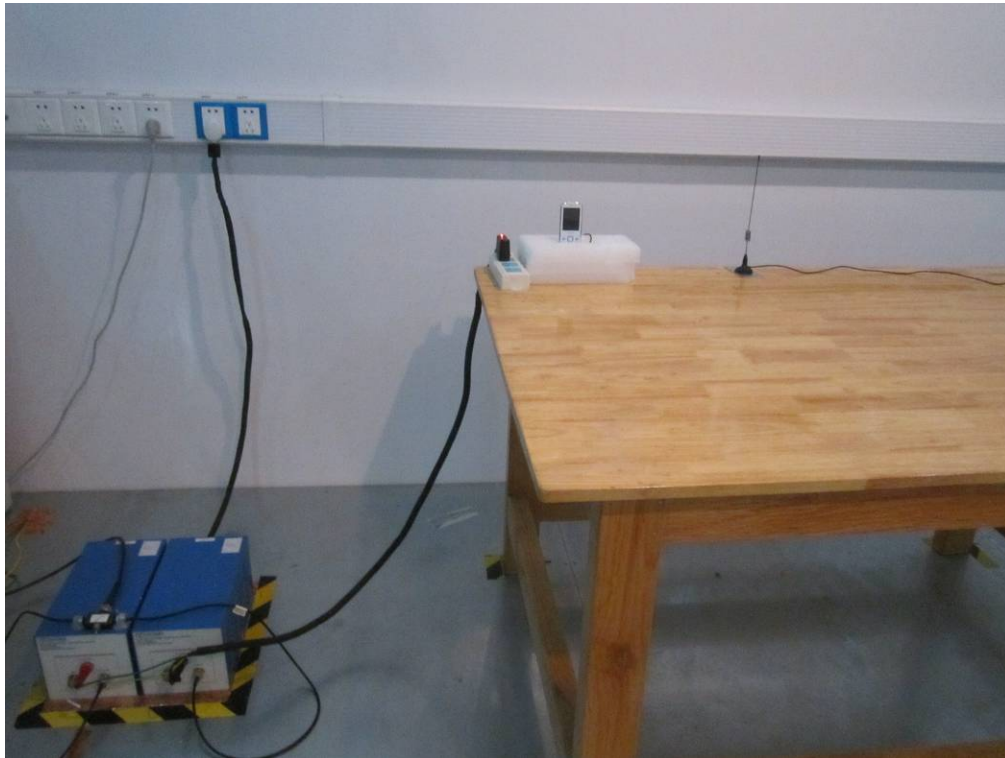
Conducted Emissions Test Setup Front View
