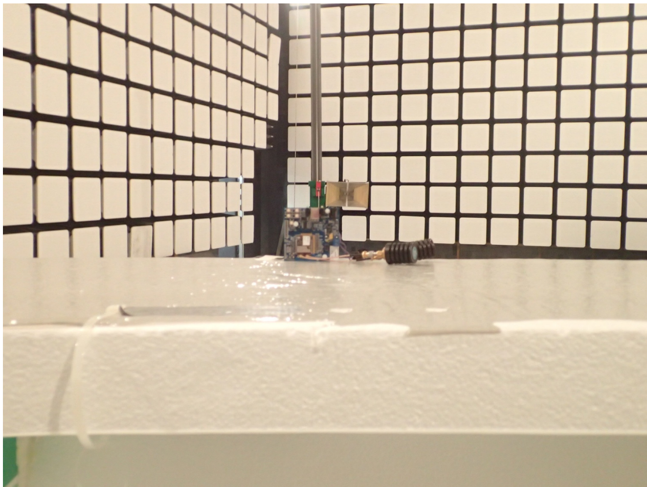
Radiated Emissions @ 3 m, Orthogonal Position 3
