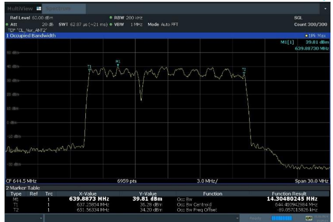
Plot 8-4. Occupied Bandwidth Plot (n71_2C_5M+10M_16QAM - High Channel, Port 2)
