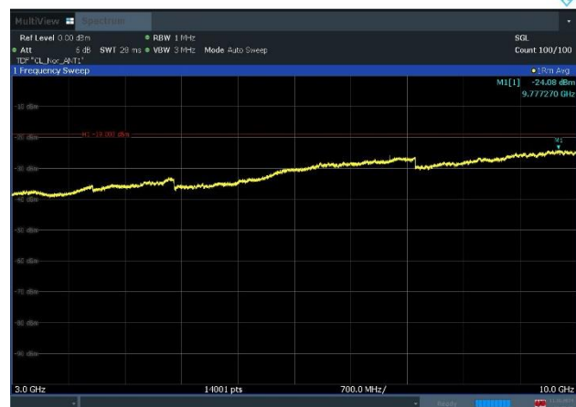
Plot 8-30. Conducted Spurious Emission Plot 3 GHz to 10 GHz (n71_2C_5M+10M_QPSK - Mid Channel, Port 1)
