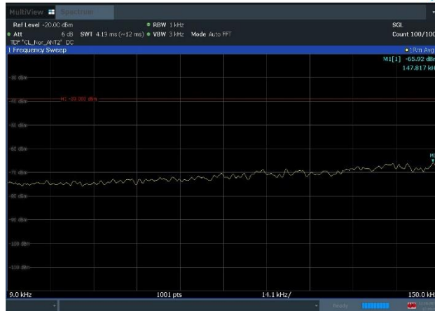
Plot 8-44. Conducted Spurious Emission Plot 9 kHz to 150 kHz (Multi band operation n71_2C_5M+10M + n29_1C_5M + n26_1C_5M_QPSK, Port 2)
