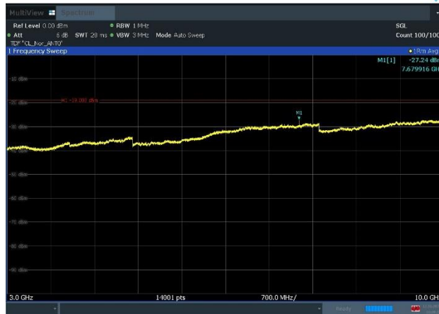
Plot 8-43. Conducted Spurious Emission Plot 3 GHz to 10 GHz (n71_2NC_5M+10M_QPSK – Mid Channel, Port 0)
