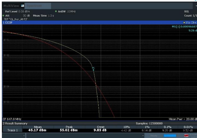
Plot 8-9. Peak To Average Power Ratio Plot (n71_2C_5M+5M_QPSK - High Channel, Port 3)
