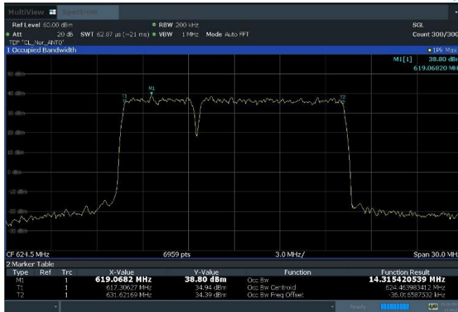
Plot 8-3. Occupied Bandwidth Plot (n71_2C_5M+10M_QPSK - Low Channel, Port 0)
