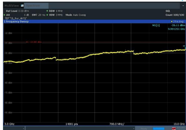
Plot 8-36. Conducted Spurious Emission Plot 3 GHz to 10 GHz (n71_2NC_5M+5M_QPSK – Mid Channel, Port 2)
