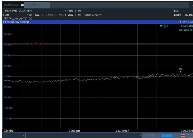
Plot 8-31. Conducted Spurious Emission Plot 9 kHz to 150 kHz (n71_2NC_5M+5M_QPSK – Mid Channel, Port 2)
