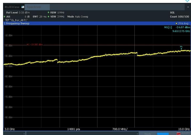
Plot 8-24. Conducted Spurious Emission Plot 3 GHz to 10 GHz (n71_2C_5M+5M_QPSK - Mid Channel, Port 1)
