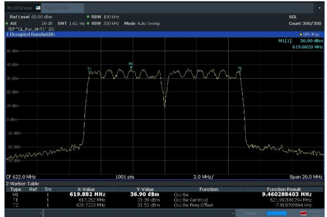
Plot 8-2. Occupied Bandwidth Plot (n71_2C_5M+5M_16QAM - Low Channel, Port 1)
