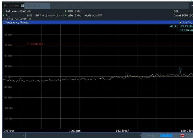
Plot 8-19. Conducted Spurious Emission Plot 9 kHz to 150 kHz (n71_2C_5M+5M_QPSK - Mid Channel, Port 1)
